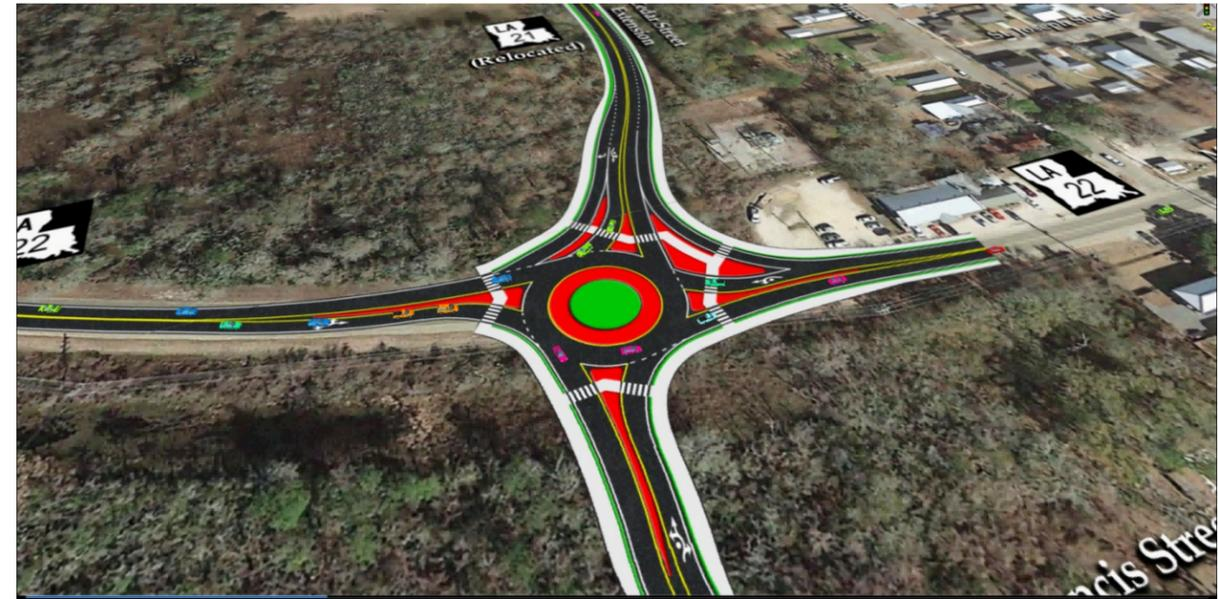
Figure 38. Vissim model of the proposed roundabout at LA 22 and the new LA 21
